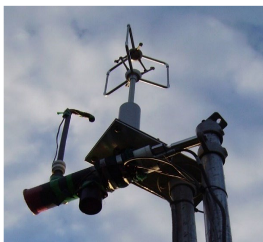
Figure 10. Images showing an eddy covariance flux tower (left); and a drone (right). Source adapted by Garfield Giff, (2025), Landscape Carbon Workshop, Yellowknife, NT [Workshop presentation].
