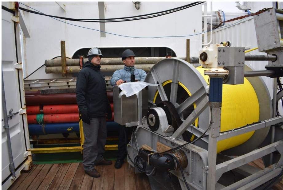
Figure 6.6 Photograph showing MiniROV winch and tether. Winch was operated manually using control box. Instructions were communicated via hand-held radio from the control room.
