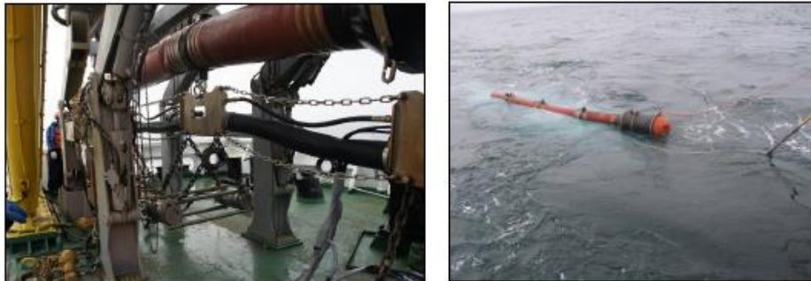
Figure 2. Photograph showing the airgun array prior to deployment with the guns visible (left). The airguns were suspended 6 meters below the surface using a large float (right).
