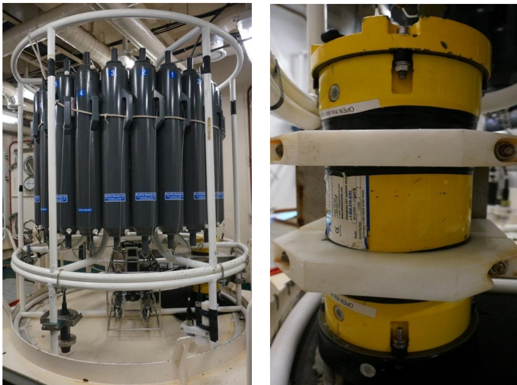
Figure 9.2. Hydrographic observation equipment. Left: SBE911plus CTD profiler and rosette water sampler. Right: 300 kHz RDI lowered ADCP.
