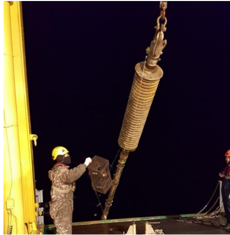
Figure 10.4. A net trap was tied to the top of the weight of gravity core, so that the net trap could rest on the seafloor in an attempt to collect seafloor fauna.
