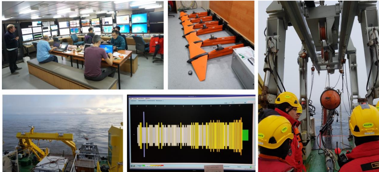
Figure 2.2. Selection of photos taken during the MCS program. From top left: MCS survey control room in the Main Dry Lab of Araon; Birds used to control the depth of the streamer; Airgun system being deployed; Airgun system in active survey; Bigshot display to monitor noise distribution on the streamer for quality control purposes.
