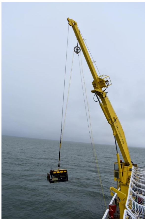
Figure 6.4 Image showing the MiniROV being deployed. The tether is routed through a turning block suspended below the crane.
