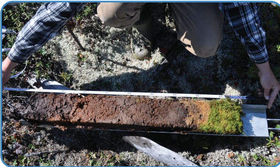
Figure 2. A peat core used to reconstruct the wildfire and metal deposition history at one of the study bogs. (Credit: Nicolas Pelletier)
