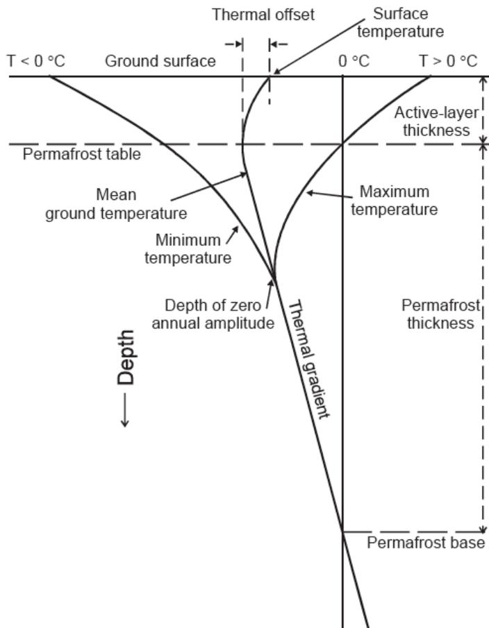
Figure 3. Typical ground temperature profile in a permafrost area (Burn CR. 2004). The thermal regime of cryosols. (In *Cryosols: Permafrost-affected Soils*, Kimble JM (ed.). Springer-Verlag: Berlin, Germany; 391-413.)
