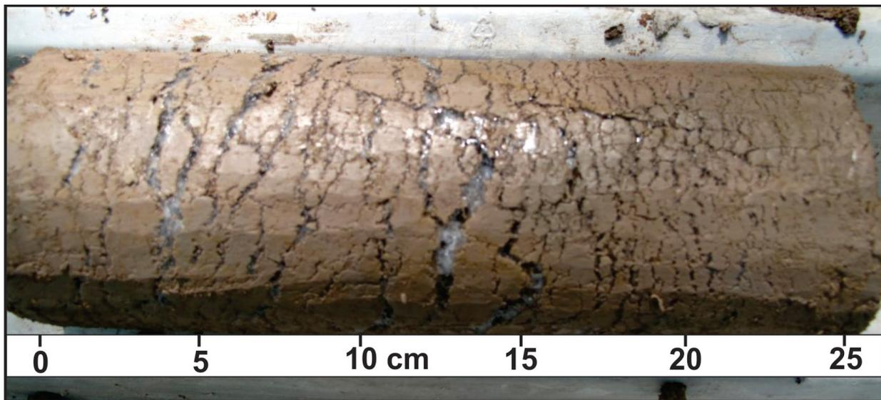
Figure 5. Permafrost core of silty clay with abundant segregated ice lenses from the Yellowknife area.
