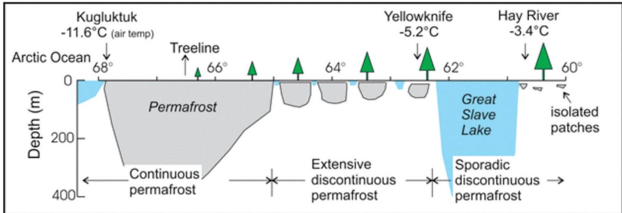
Figure 2. Permafrost thicknesses and mean annual air temperatures along a north to south transect from Kugluktuk, Nunavut to Hay River, NWT (Adapted from Brown RJE. 1970. Permafrost in Canada. University of Toronto Press, 234 p).
