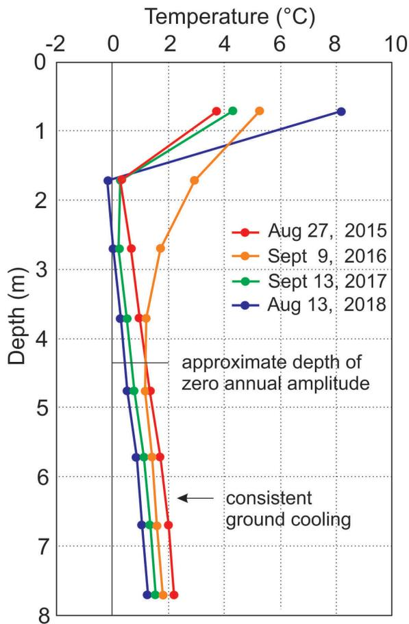
Figure 25. Ground temperatures recorded at a drained lake site indicating consistent ground cooling at depth, but an absence of permafrost formation since the lake drained.
