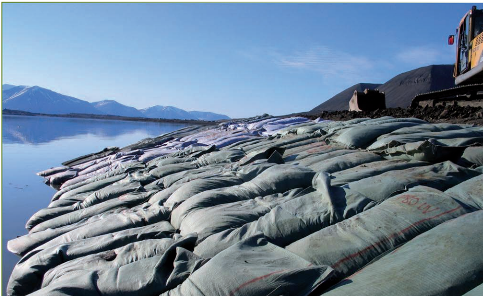
The testing of a new geosynthetic material for sandbagging coastal sites in danger of erosion (photo: SINTEF, Trondheim).
