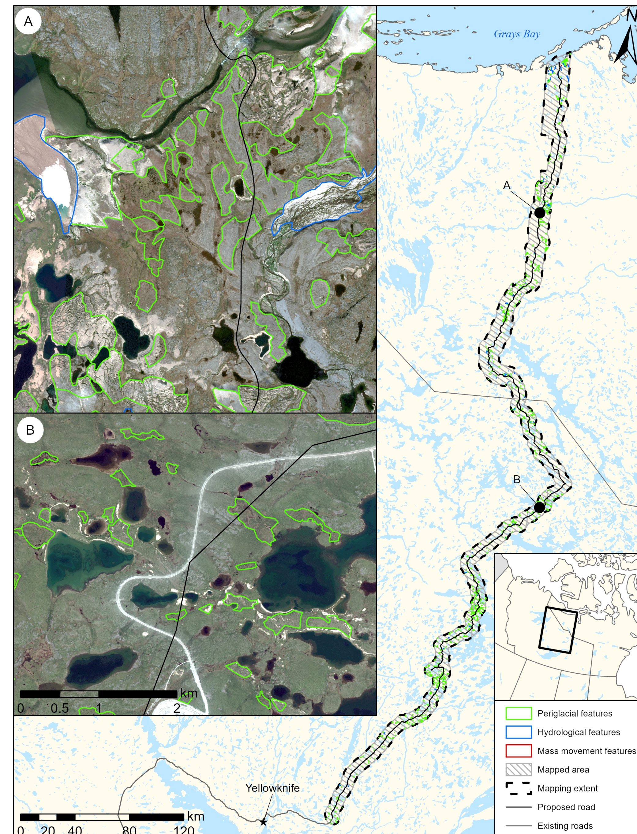
Figure 4. The study area was developed according to a 5-km buffer of the centre lines of the road corridors proposed for the region. We acquired available satellite image and then tasked the satellite constellation to fill in gaps in image coverage.
