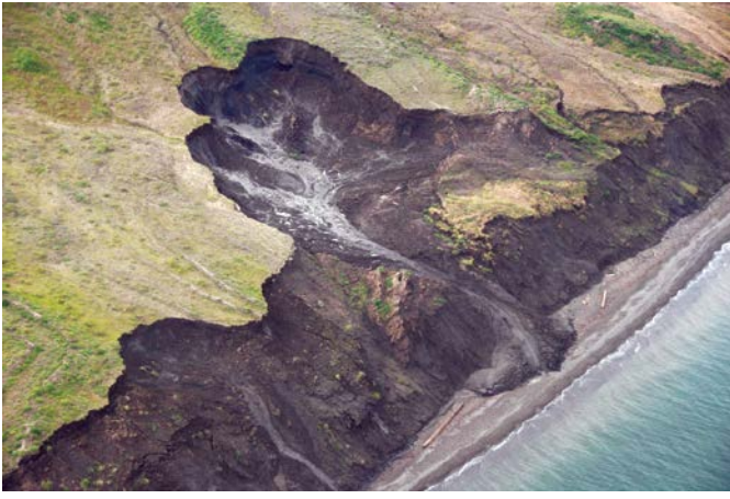
FIGURE 5: Aerial photograph of retrogressive thaw slump along the Beaufort Sea coast, YK, generated by the thawing of ice-rich sediment. Photo courtesy of N.J. Couture.
