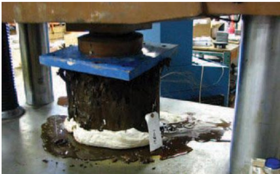
Figure 5. Laboratory load testing of decayed pile top
